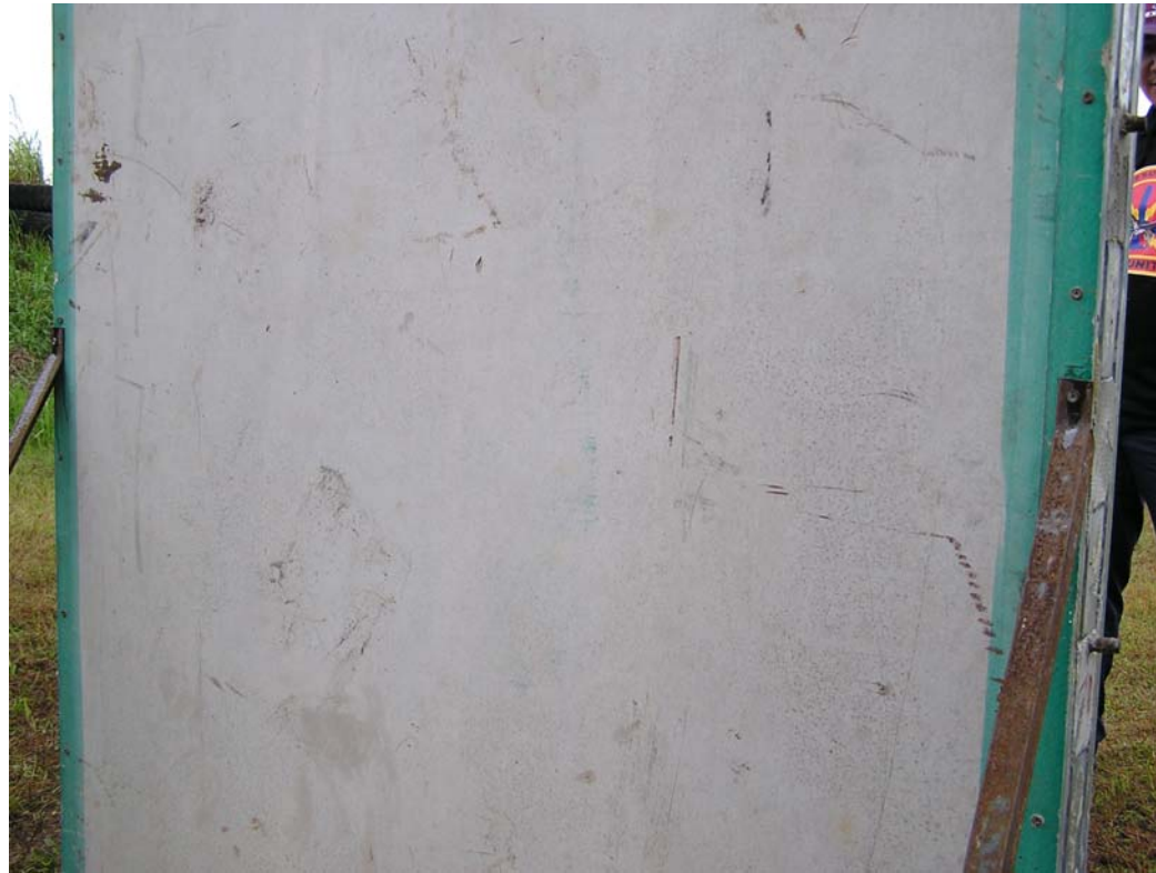
Test 9mm , 45 & M16 at 25mts Back of Panel
