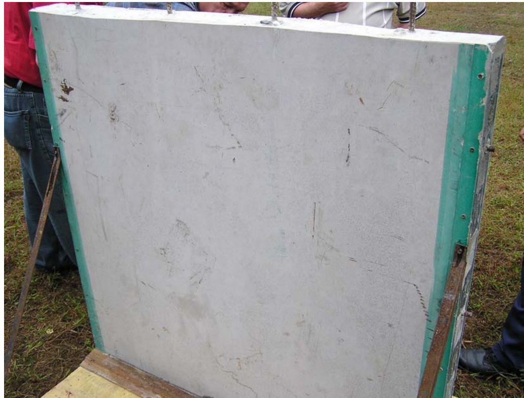
Rear of panel after 9mm & 45 test no damage
