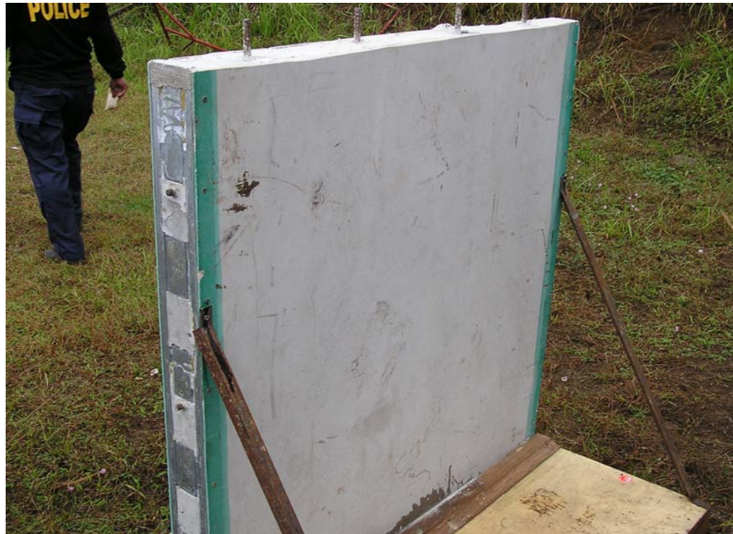
Rear of panel after 9mm test no damage
