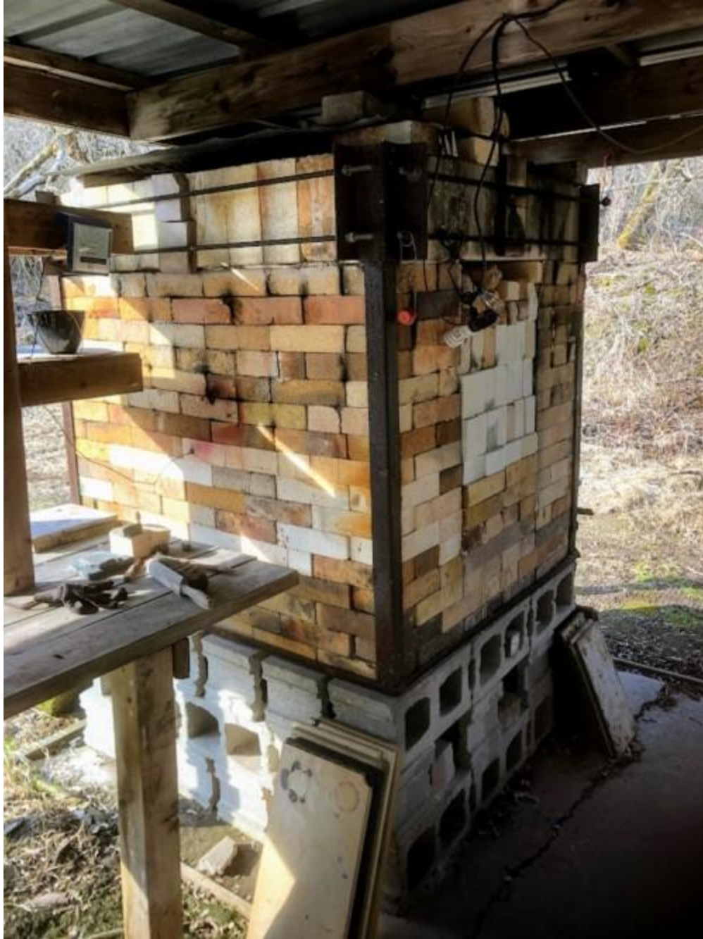
The small kiln at the farm/ it has fired to cone 7 in 4 hours
