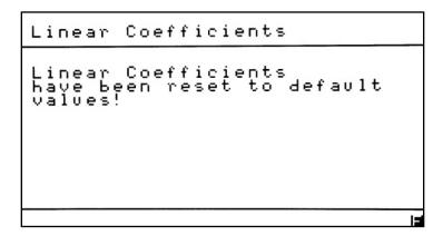
**NOTE:** After resetting Linear Coefficients, the analyzer must be zeroed and spanned before further use.
