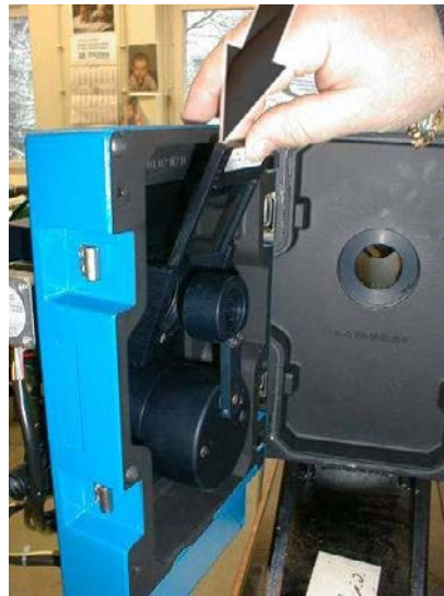
Fig. 8.4: Insert the test filter into the device
