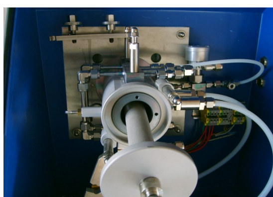
Figure 9: Dismounting of the filter housing cover
