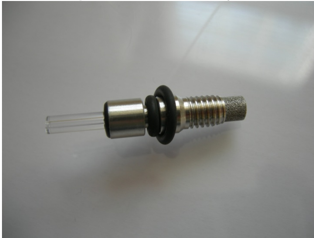
Pointed Portion Of Orifice Inserts Into Prefilter Assembly & 2 O-Rings Required On Orifice Figure 20: Orifice and Suction Tube
