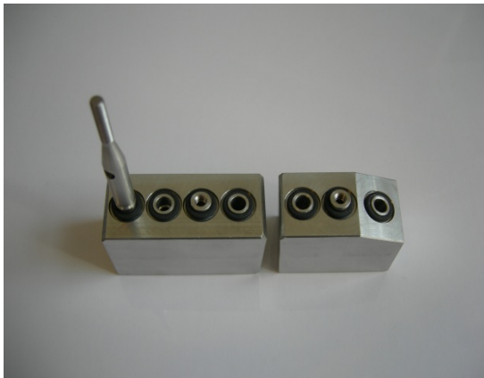
Figure 18: Dilution block with critical orifice, eductor, O-ring seals and tool
