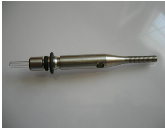
Figure 18: Dilution block with critical orifice, eductor, O-ring seals and tool
