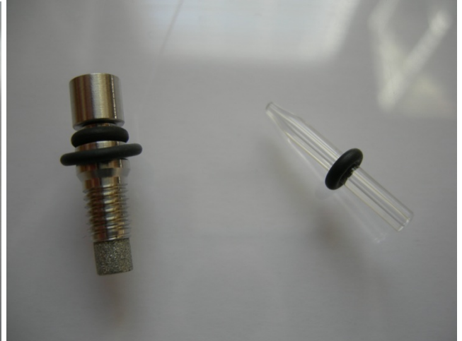
Pointed Portion Of Orifice Inserts Into Prefilter Assembly & 2 O-Rings Required On Orifice Figure 20: Orifice and Suction Tube
