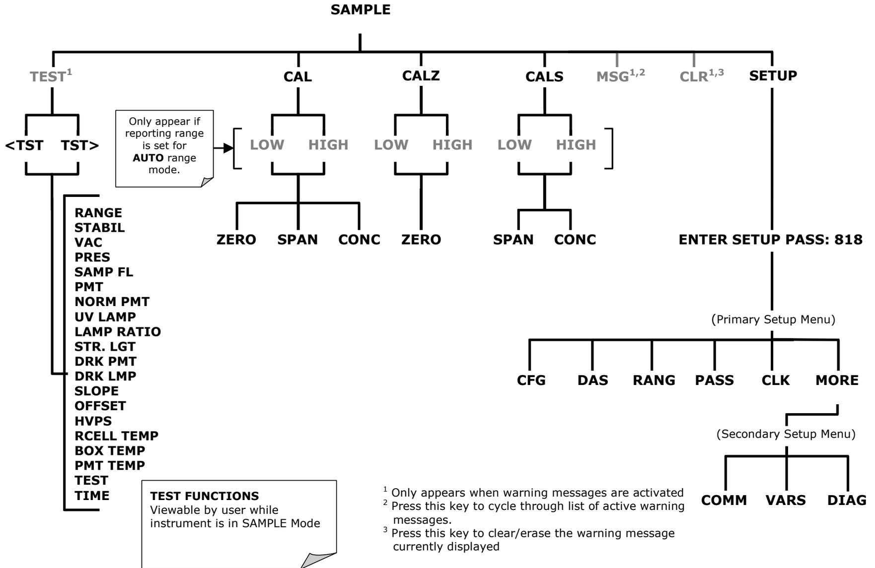
**Figure A-2: Sample Display Menu - Z/S Valve Option installed**
