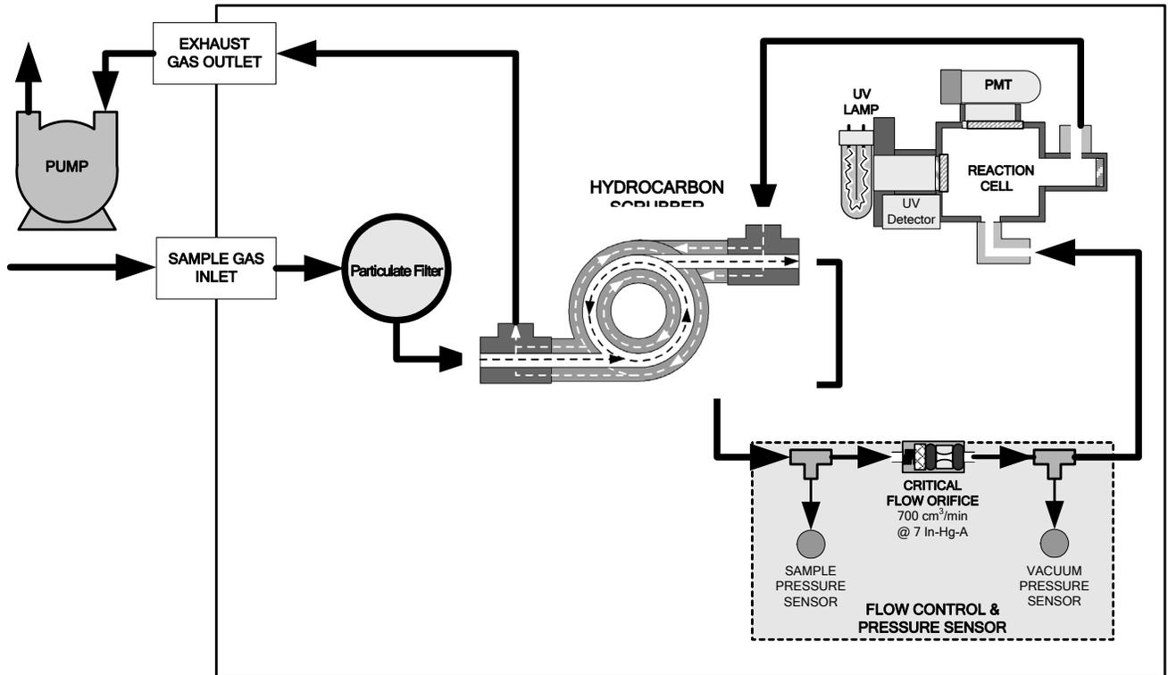
Figure 5-4: T100H Internal Pneumatic Diagram with Hydrocarbon Scrubber Installed
