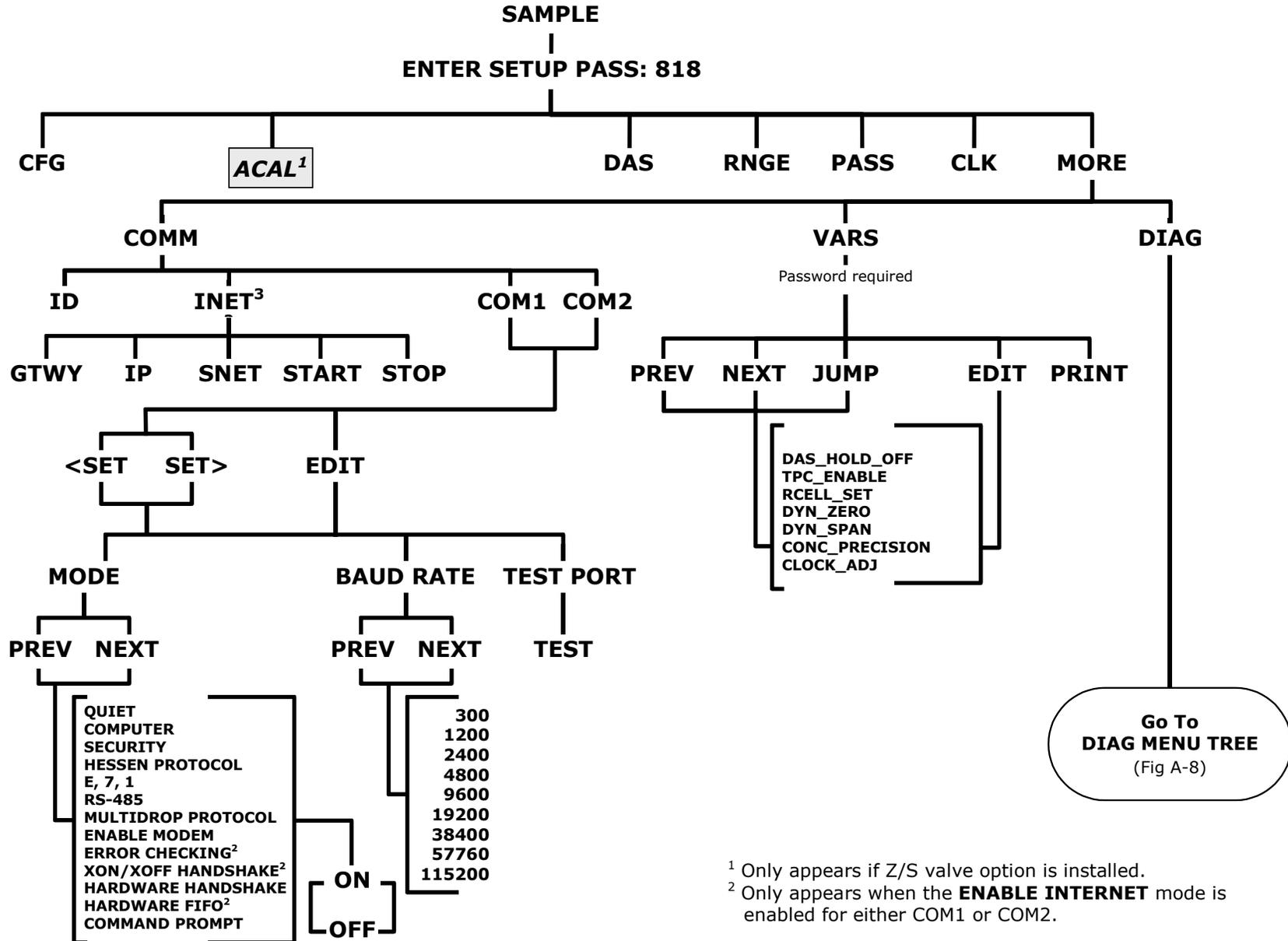
Figure A-5: Secondary Setup Menu (COMM & VARS)
