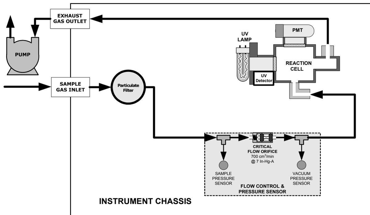
Figure 9-2: Pneumatic Diagram of the T100H – Base Configuration
