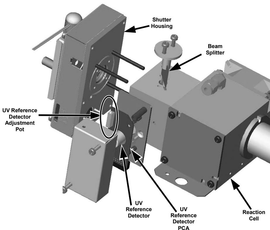
Figure 10-4: Location of UV Reference Detector Potentiometer
