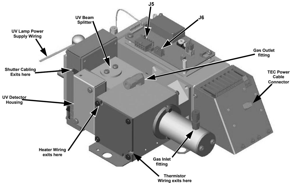
**Figure 10-2: Sensor Module Wiring and Pneumatic Fittings**
