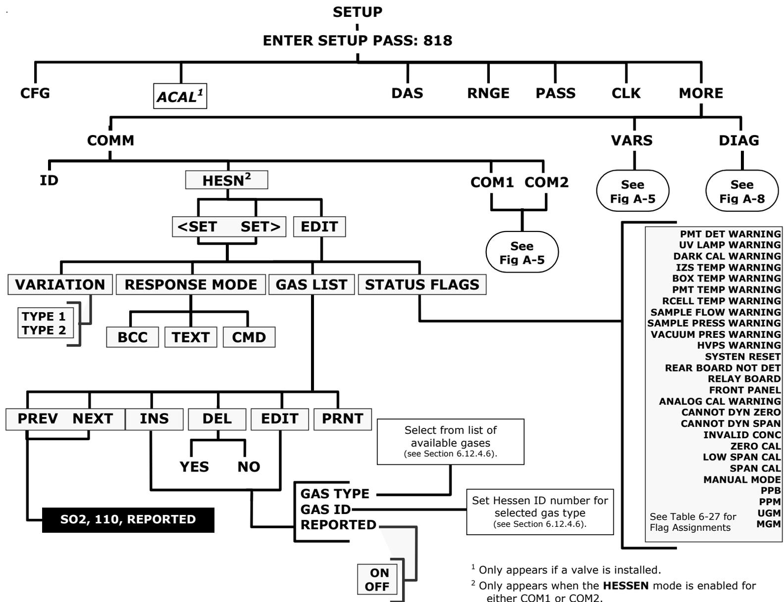
Figure A-7: Secondary Setup Menu - HESSEN Submenu
