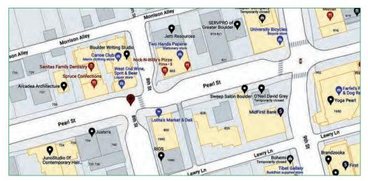
A Google map view of the Eighth and Pearl development block in Boulder, CO shows how the project optimized the available space of the street right-of-way by introducing "bump-outs" at the intersection, which facilitated both on-street parking and available outdoor seating space.
