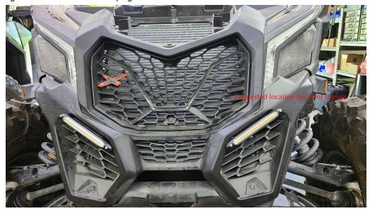
**Eyebrow signal light option.** Replace the accent lights and connect the original plugs. (Search Youtube for Can-Am X3 eyebrow installation videos). Carefully route the wires to the cables marked "Right front signal & Left front signal" and connect the small plugs.
