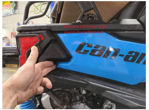
At the rear of the machine remove the colored bed side covers to expose the tail light plugs as shown. Route the cable to the left tail light plug then across the rear to the right tail light following the existing wire harness making sure to avoid the hot exhaust. Unplug the old cables and plug in the new BX3 cables. On the left connect the new plug with the single wire to the old plug.
