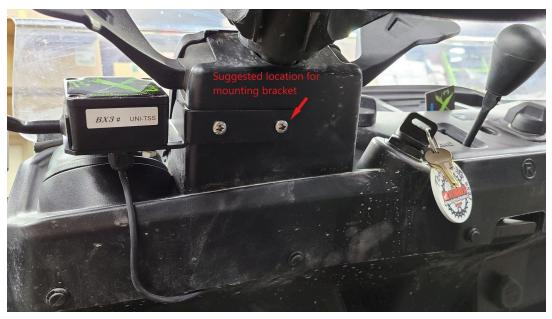
Replace the top cover. Route the cable along the steering column to the control box and plug it into the plug marked with black heat shrink.
