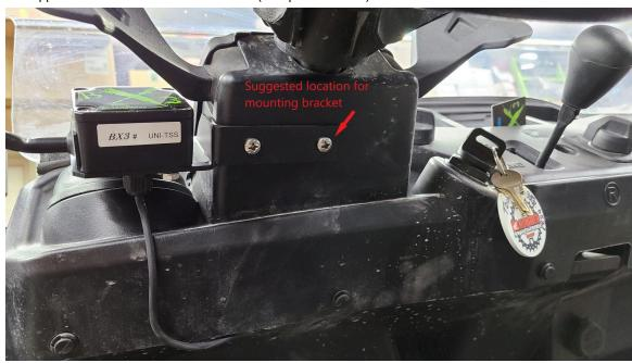
Route the cable along the steering column to the control box and plug it into the plug marked with black heat shrink.
