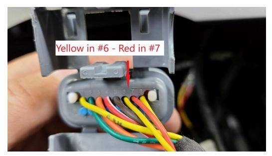
Route the wires to the cable marked "Right and Left indicators". Connect color to color. Black is not used
