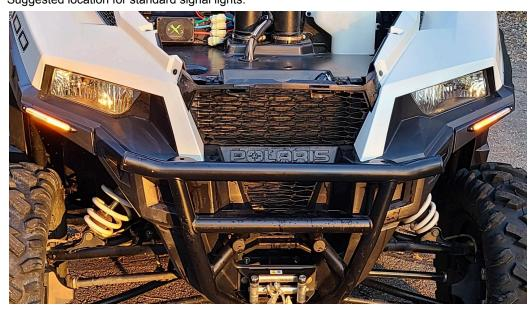
**Signal headlights with driving lights available.** Replace headlights and connect to the original plug or use the adapter cable. Connect the small plugs together.
