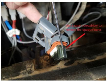
Route cable marked POA-CIC to the large plug. Remove the small seal plugs from holes 6 & 7. Insert the yellow wire in hole 6 and the red wire in hole 7. Replace the opaque cover and close the back. Route the wires to the cable marked "Right and Left indicators". Connect color to color. Black is not used
