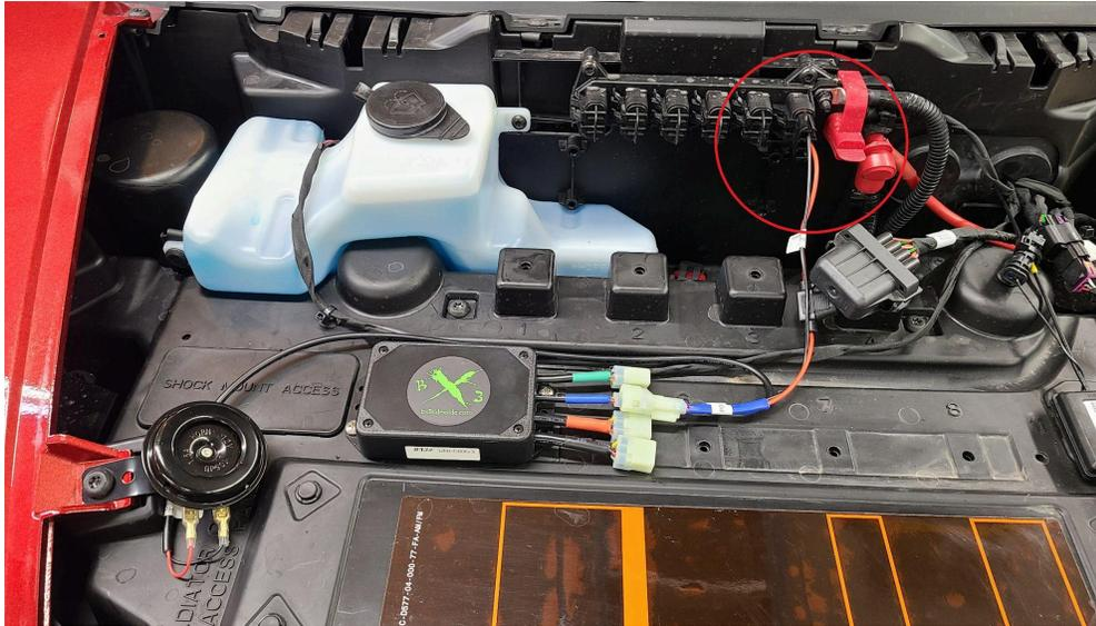
**Use cable ties to secure all cables and connector plugs.**
