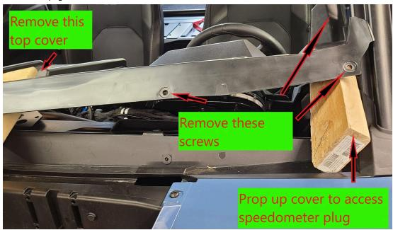
Reach in and carefully pinch the latch and unplug the large plug from the back of the speedometer.
