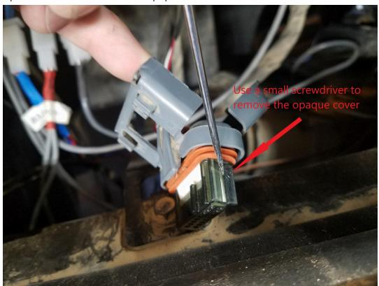
Route cable marked POA-CIC to the large plug. Remove the small seal plugs from holes 6 & 7. Insert the yellow wire in hole 6 and the red wire in hole 7. Replace the opaque cover and close the back.
