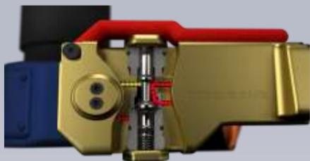
When the “Dead Man Safety Lever” is depressed, the flow of oil is diverted from the tool, preventing the tool from actuating, thus preventing injury.
