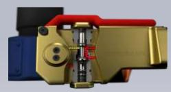
When the "Dead Man Safety Lever" is depressed, the flow of oil is diverted from the tool, preventing the tool from actuating, thus preventing injury.
