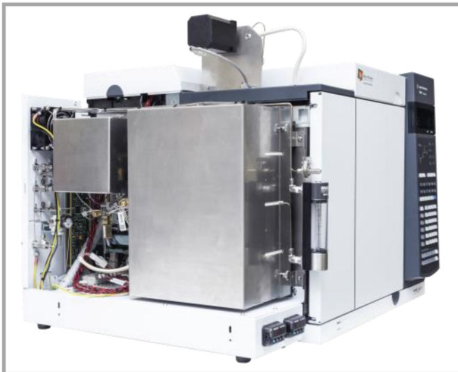
Figure Two: The heated DVLS Side Carrier
