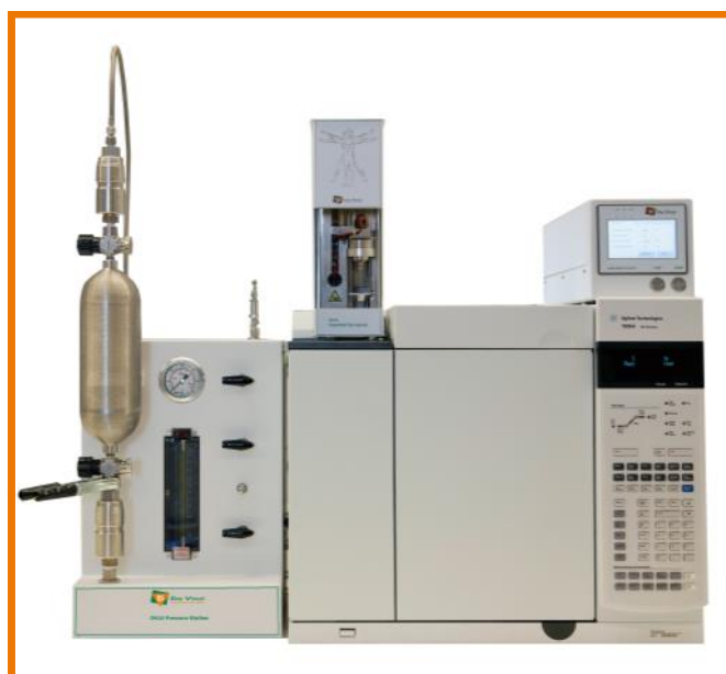
Figure One: Agilent GC & DVLS Liquefied Gas Injector
