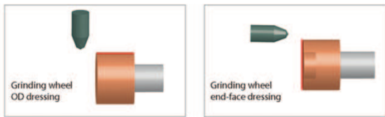
Grinding Wheel Dressing Graphic Illustration
