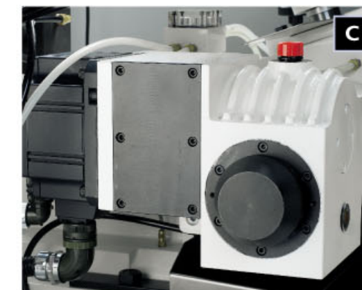
Regulating wheel is driven by AC servo motor.
