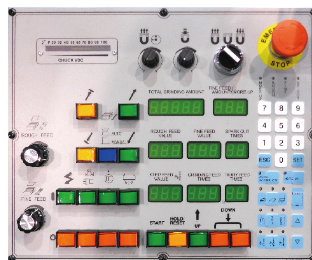
AUTOMATIC DOWNFEED AD5 (NC) CONTROL PANEL (optional)
