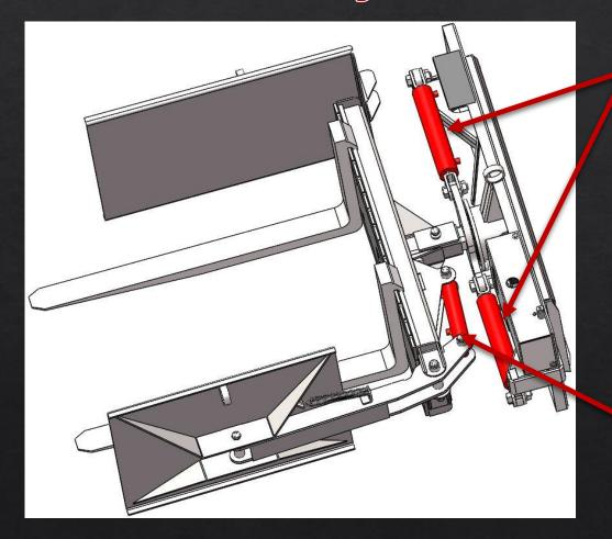
\*Clamping Fork Tool on Double Cylinder Rotating Base 1. ROTATION CYLINDERS
