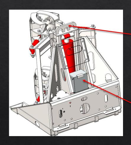
LIFTING POINT FOR PLACING POLE JACK WITH A DIGGER DERRICK TRUCK
