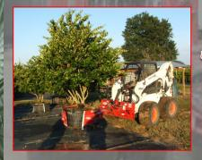
The Pot Mover attaches to any machine and can handle all types of trees.
