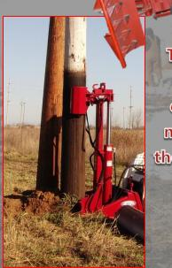
Two large 3x6 inch clamp cylinders and metal teeth on the jaws securely hold pole in place during extraction.
