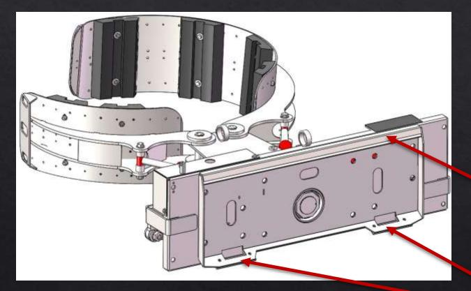
Quick attach plate has gusset on top for extra support.
