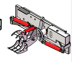
ROTATES 127° TO OPERATOR'S LEFT WEIGHT= 523.72 LBS
