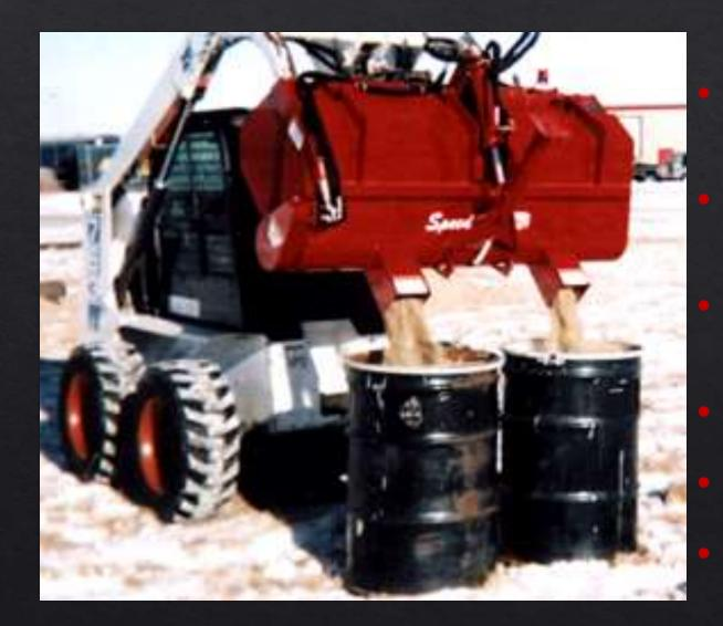
Augers are enabled only when the lid is closed engaging the sequencing valve. Conversion nozzle can be purchased to make it a single shoot unit.
