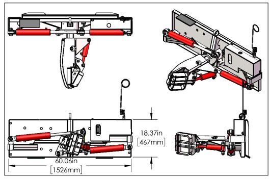
ROTATES 127° TO OPERATOR'S LEFT WEIGHT= 541 LBS
