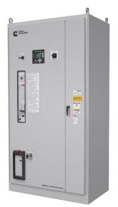
The B-Series transfer switches are suitable for use in emergency, legally required and optional standby applications. The integral automatic transfer switch control monitors both power sources, signals the generator set to start and automatically transfers the load to the alternate power source. When the preferred power source returns and has stabilized, the load is automatically transferred back.
