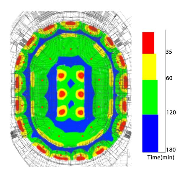
Possible to use software such as AGi32, Dialux, and others to create photometric and thermal mapping to calculate necessary amount of fixtures.
