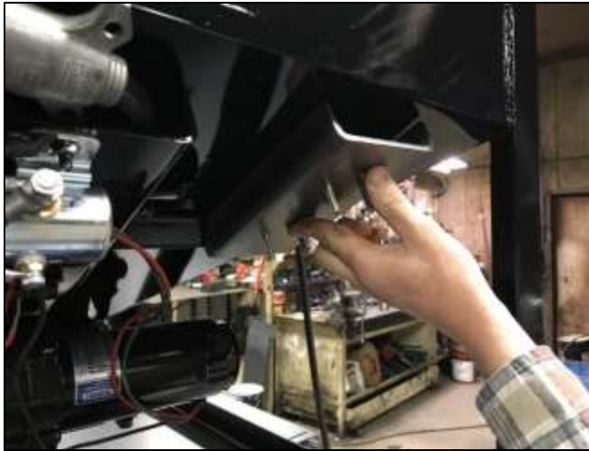
Photo 4: You may need to apply pressure in the area indicated by the thumb in the photo to force the plate flat against the bottom of the feeder. You can try using a jack positioned between the plate and the bottom runner of the feeder to accomplish this. Once properly aligned, tack weld the plate to the bottom of the sheet. Then apply stitch welds at the locations marked “Stitch” on the plate.
