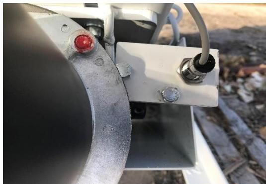
Run the new sensor wire from the caker to the pickup cab. Then place the Pierce Digital Counter Monitor on your dash in cab of vehicle.
