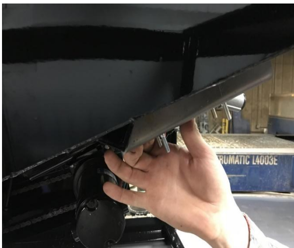
Photo 3: It will probably be necessary to tack the Vibrator plate to the point of the angle iron, on both sides of the plate. (Tack points are marked on plate.)
