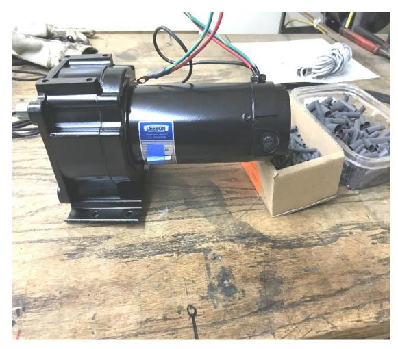
This unit runs on a 1/8 HP 12 Volt motor/gear box combo, connected to the UTV with the hot wire and an inline fuse holder, with a 20-amp fuse (provided)
