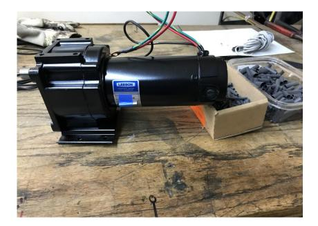
This unit runs on a 1/8 HP 12 Volt motor/gear box combo, connected to the ATV with the hot wire and an inline fuse holder, with a 20-amp fuse (provided)
