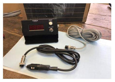
Our Digital counters are a small Plastic box that we've built brackets around that will be mounted in the cab of your pickup, typically on the dash. They plug in to your vehicle's power point and have a digital read out display with a simple and clean design. This counter will only count revolutions, so you will need to calibrate it to your feed output
