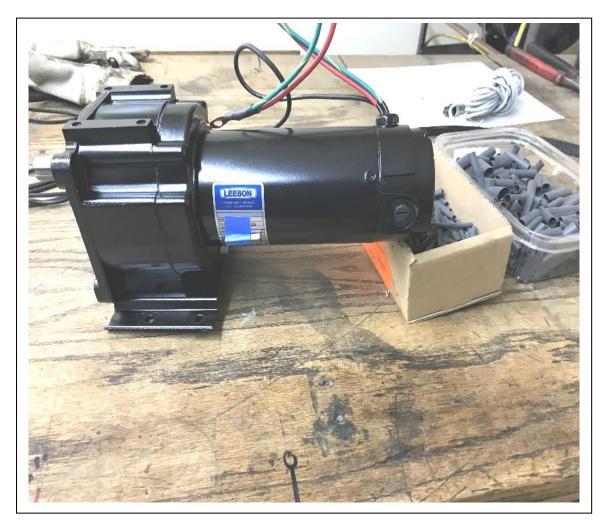
This unit runs on a 1/8 HP 12 Volt motor/gear box combo, connected to the UTV
