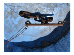
5. Turn your tub right side up again. Set it on Blocks or pallet. Place a chain through each hole with your bar inside the tub. You will then need to drill 2 small holes in the rim of the tub to be able to suspend your anchor with wire to each side of your tub. The bar should be suspended about 4 inches above the bottom of the tub.
