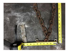
4. You will need a chain anchor for each tub. (We have these anchors for sale, cost \$13.00 per tub.) Anchors are a 6 inch piece of Rod with 3 welded eyes, one on each end of the rod and one on the center of the rod, and 22 inches of 5/16" chain.
