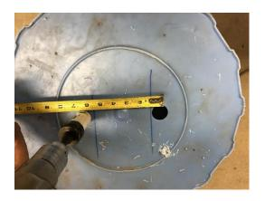
3. Using a 1 1/8" hole saw drill a hole on each side of your spacer mark.
