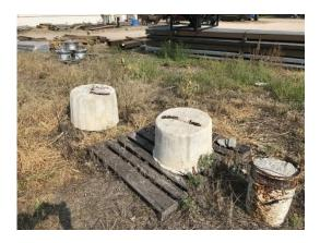
9. Once the concrete has cured in the tubs, remove the concrete from the tubs.
