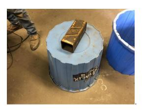
2. Turn the tub upside down, Use a 4"X4" block to mark your hole spacing.
