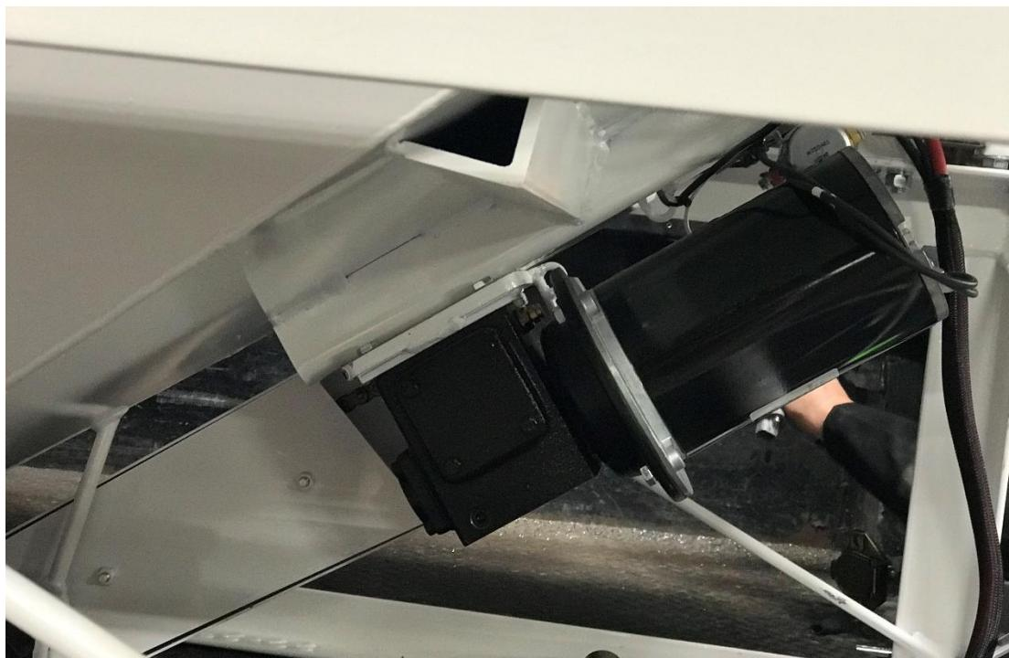
You will need to install the brass breather plug before you bolt the motor to the gear box.
