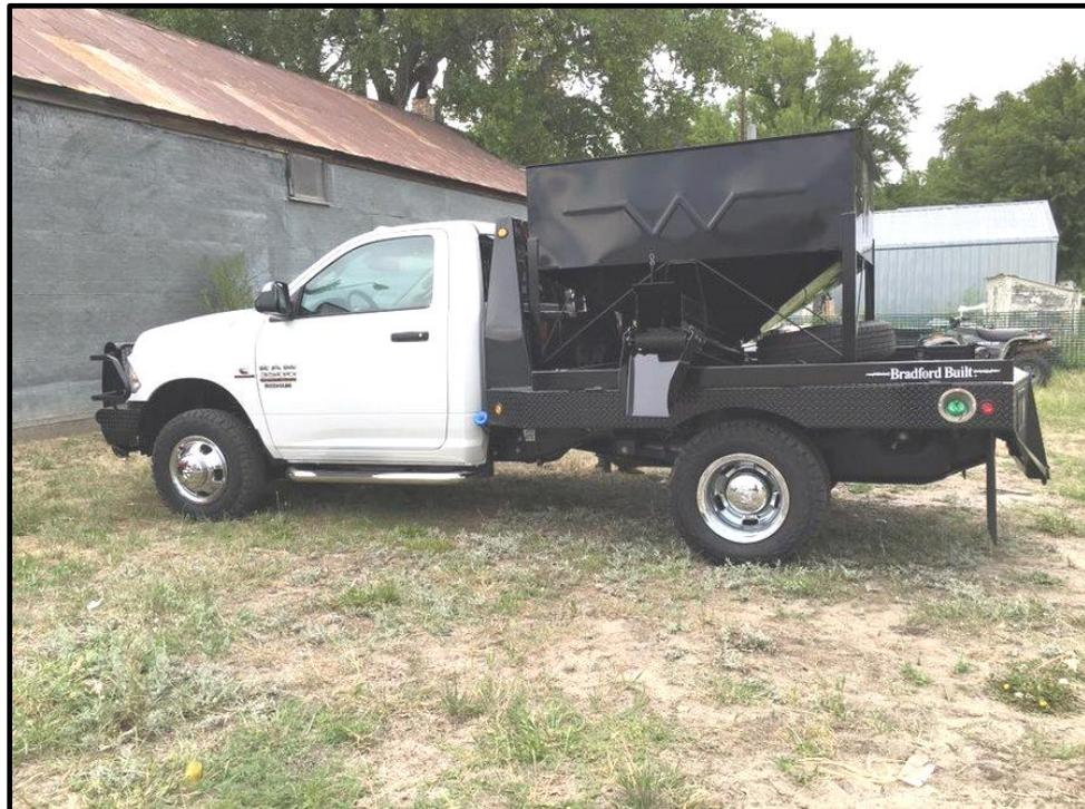
Take the caker off of the flatbed and flip it over. This will make it much easier to replace and install the new motor & gearbox system.
