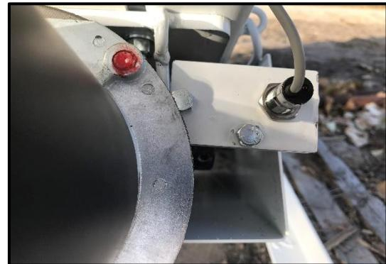
Run the new sensor wire in both the caker-side wiring harness & the pickup cab.
