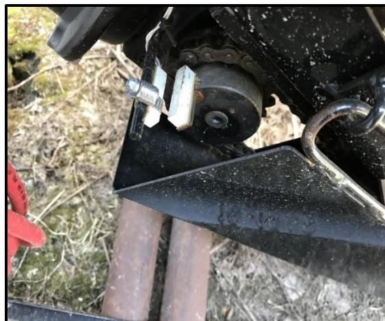
Mount the sensor with the included brackets around the post that you removed the magnet sensor from.
