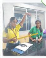
Activity- Finding mass of a given body using metre scale by principle of moments.
