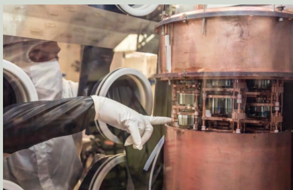
[The installation of a cryostat module in the Majorana Demonstrator. (Image Credit: Sanford Underground Research Facility)]
