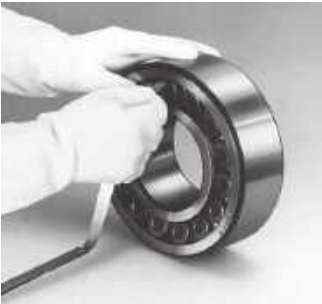
Fig. 1 Clearance Measurement Point (Bearing Outside Diameter: Less Than 200 mm)
