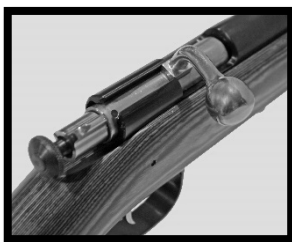
Bolt handle fully forward and at the mouth of the chamber
