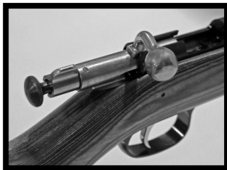
Bolt handle up and fully to the rear of the receiver.
