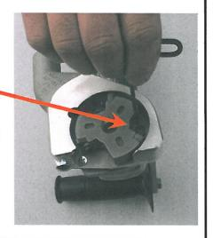
Instructions for adjusting the depth of cut on the butt surface
