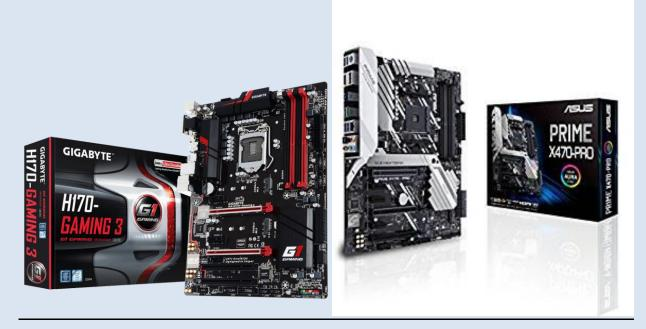
The most important thing you need to check is that motherboard socket is right for your chosen CPU. You can check what socket the CPU requires on Intel's or AMD's web page. For example, Intel's most popular socket is LGA1151 and AMD, on their newest processors, uses AM4 socket.
