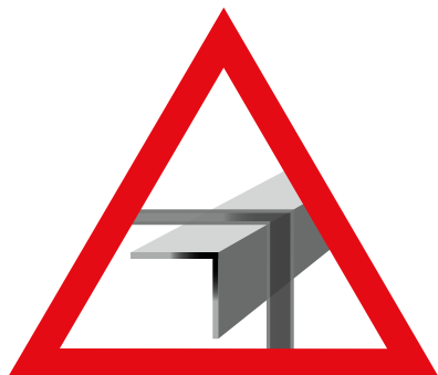
Global Sharp Edge symbol— Radius as sharp as 0.25 mm (0.0098")
