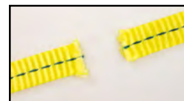
Failure due to sharp edge conditions
