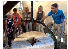
how it operates were explained. The giant stone for grinding corn was in the process of being replaced and we learned that it took 4 years to locate the perfectly-sized French Buhr stone. This stone is very hard and can last for over 100 years and is carved specifically to grind the grains. There is also another grinding stone for wheat. The new corn wheel was due to return to service in 1-2 weeks.
