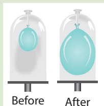
Figure 8.17 A balloon in a jar expands when air in the jar is removed.
