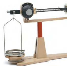
Figure 3.4 Simple beam balance used to measure mass
