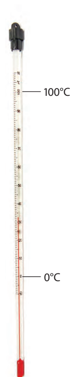
Figure 8.18 A glass thermometer with a Celsius scale
